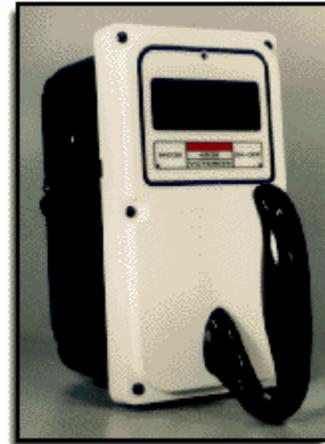
The only controls present on the basic instrument are an ON/OFF button and a MODE button. No other controls are necessary because the instrument is both auto-ranging and auto-zeroing.
